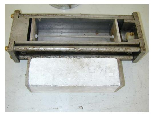
Fig. 9 - Restrained expansion specimen (UNI 8147).
