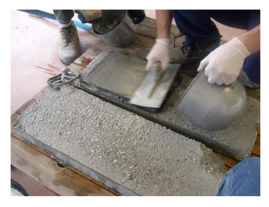
Fig. 5 - Concrete substrate for bond strength test (UNI EN 1766).
