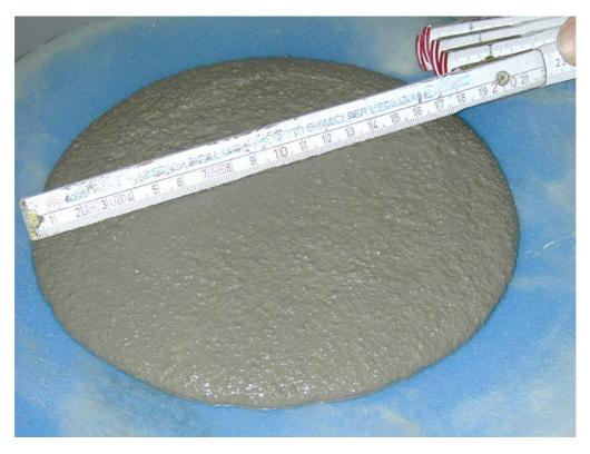
Fig. 4 B - Flow table measurement for flowing mortar.
