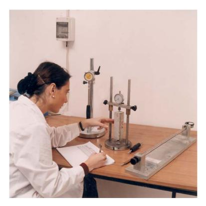
Fig. 11 - Shrinkage measurement (UNI 6687).
