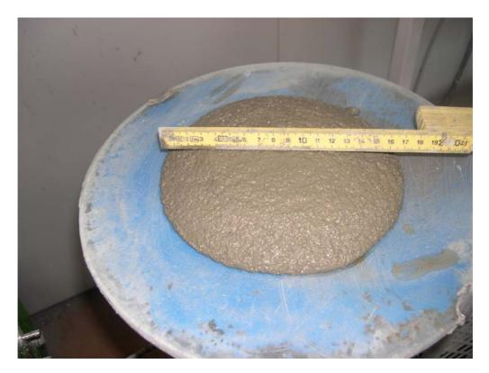
Fig. 4 A - Flow table measurement for tixotropic mortar.
