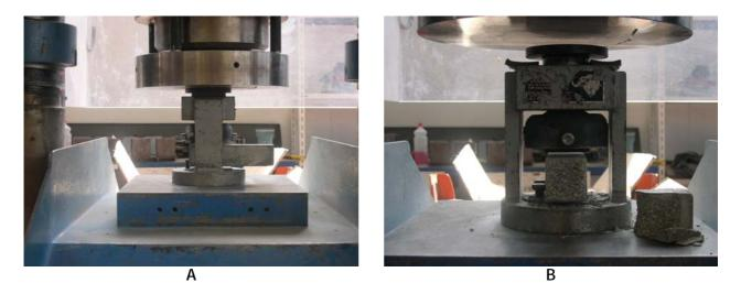
Fig. 14 A-B - Compressive strength test on mortar specimen (UNI EN 196/1).
