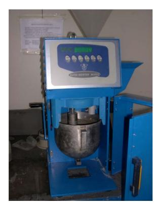
Fig. 1 - Mortar mixing apparatus UNI EN 196/1.
