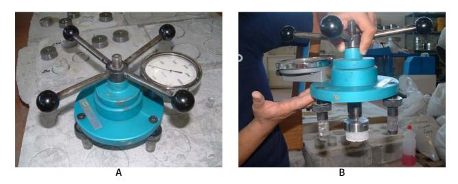
Fig. 7 A-B - Pull-Off apparatus for bond strength measurement (UNI EN 1542).
