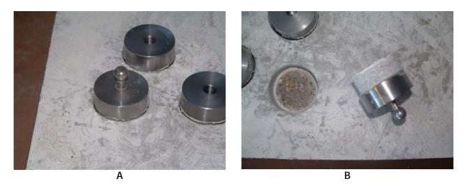
Fig. 8 A-B - Specimens for pull-off test (UNI EN 1542).
