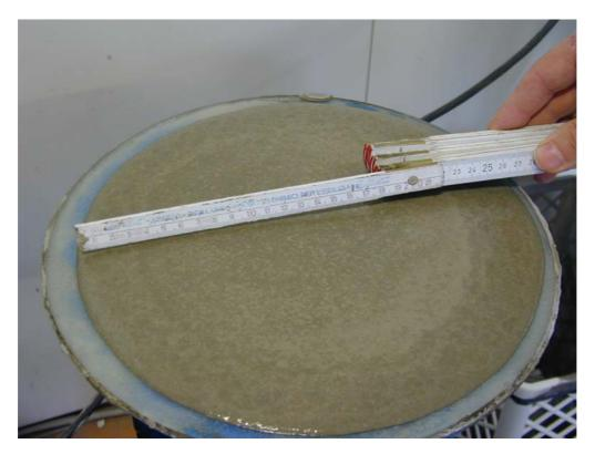
Fig. 4 C - Flow table measurement for self leveling mortar.
