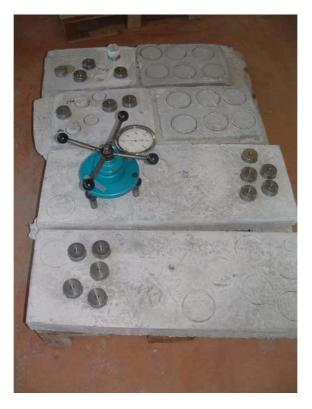
Fig. 6 - Bond strength test by pull-out (UNI EN 1542).
