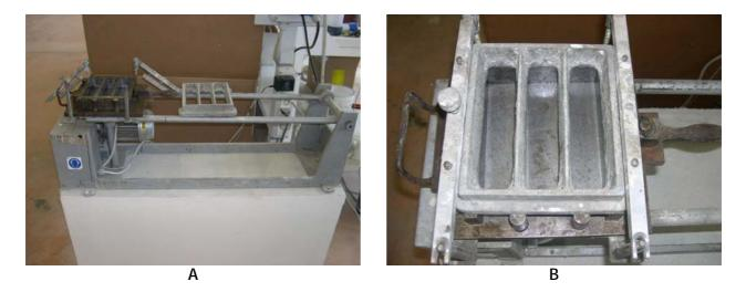
Fig. 12 A-B - Casting apparatus for mortar specimens(UNI EN 196/1).
