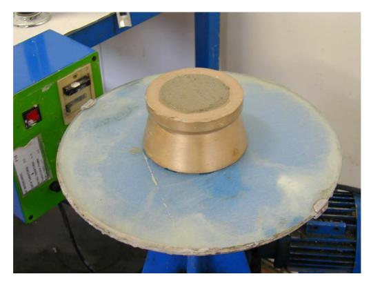
Fig. 3 - Mortar come for flow test (UNI 7044).
