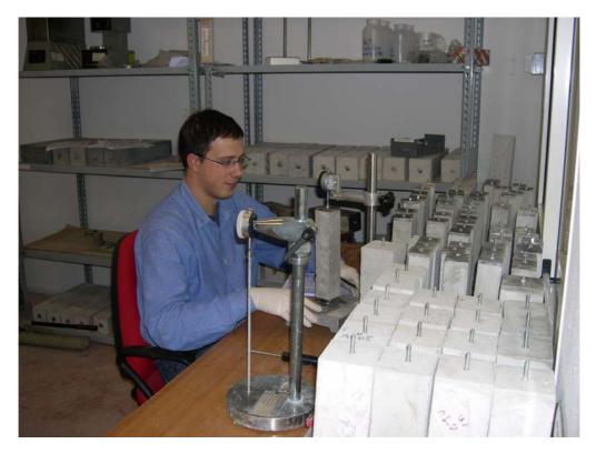
Fig. 10 - Restrained expansion measurement (UNI 8147).
